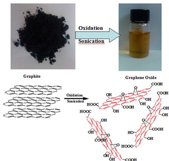
Figure 3. Schematic illustration of graphite by oxidation. [Color figure can be viewed in the online issue, which is available at wileyonlinelibrary.com .]
